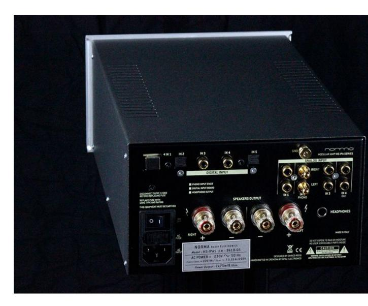
The connectors are all high quality and gold plated. There are four pairs of analogue RCA inputs, one pair of which connects to the optional phono stage, as well as USB, Toslink and S/PDIF for the optional DAC. The headphone socket is also on the rear panel - the matching amplifier is another optional extra. The Norma remote control is a chunky aluminium lump with a large array of buttons to cover every function. The buttons are a little small but it works perfectly well.
